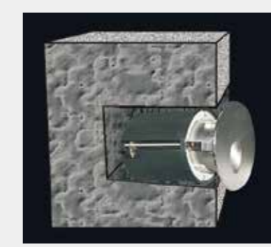
Installation with clips embedded into sleeve, fix on the concrete wall
