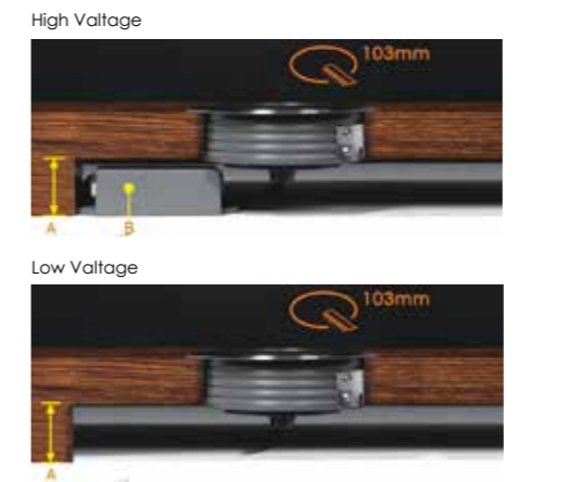
A: Minimum space for external driver is 48mm B: External IP67 water-proof box for driver of high voltage · RGB · RGBW type
