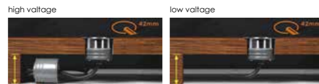
A: Minimum space for external driver is 48mm B: IP67 120V/240V/24V&RGB 24V external input driver
